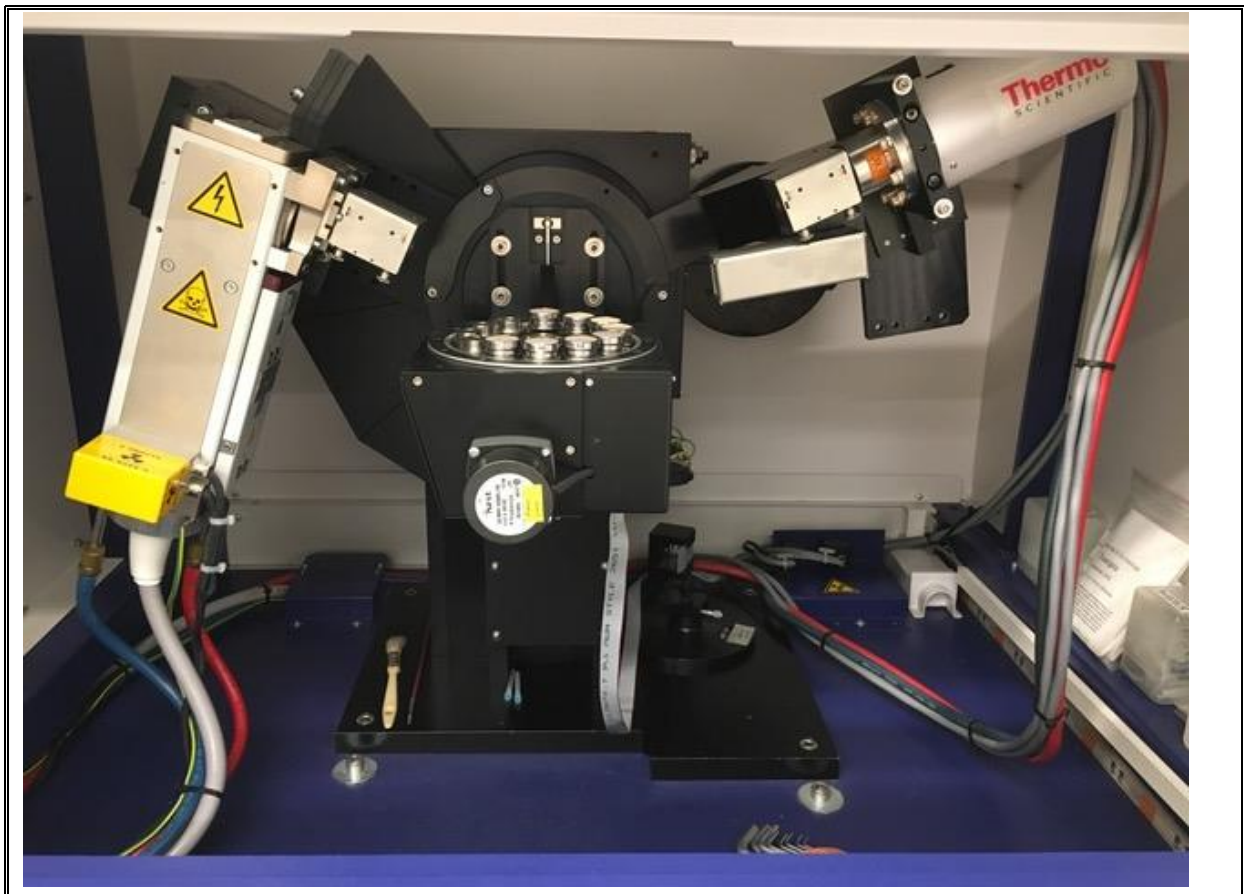
Figure 8. X-ray diffraction machine (ARL X'TRA X-RD) at Historic Environment Scotland Conservation Science Facility.
