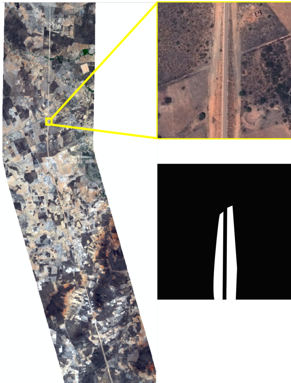
Figure 9. A sample image of Railway Erosion Dataset and a zoomed region with ground-truth. Legend—White: Erosion areas. Black: Non-erosion areas/Background.
