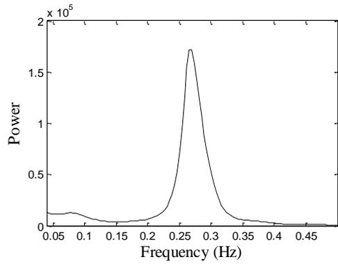
Figure 2: Power Spectral Density (PSD) using AR
