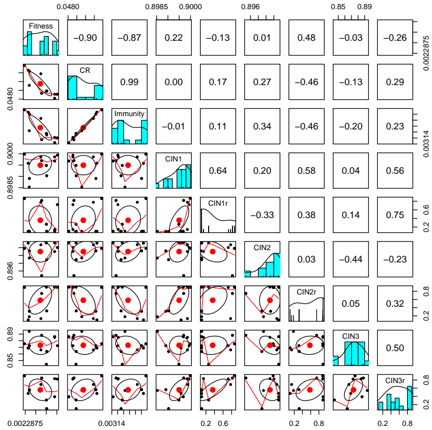
Fig. 7. PSO parameter correlations: one-stage. Variables under optimisation along the diagonal. Bottom left shows scatter plots of pairs of variables. Upper right side shows the corresponding correlation values. X-axes labels alternate top and bottom. Y-axes labels alternate on left and right.
