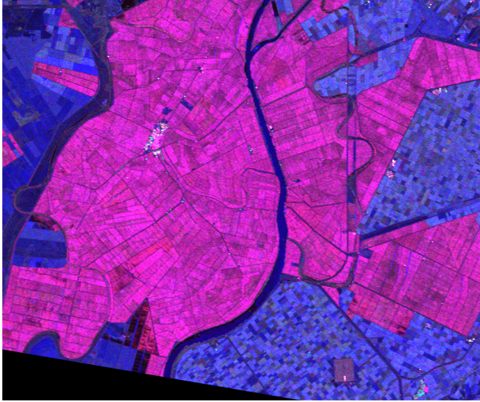
Fig. 1. Rice fields in the south of Spain (Test site 1). Quad-Pol RADARSAT-2 image acquired the 02/08/2014. Blue: \sqrt{\lambda} \cos(\underline{\alpha}) , Red: \sqrt{\lambda} \cos(\underline{\alpha}) \sin(\underline{\beta}) , Green: \sqrt{\lambda} \sin(\underline{\alpha}) \sin(\underline{\beta}) . See (9).
