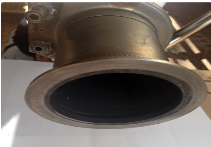
Figure 1: Air supply ducting of a B737 aircraft [35].
