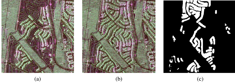
Fig. 5. UAVSAR images (in Pauli decomposition) on April 23, 2009 and May 11, 2015. (a) before change. (b) after change. (c) ground truth where white color is change and black color is no-change.
