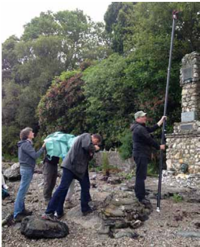
Figure 78: Using a 'magic pole' telescopic rod to photograph hard-to-reach sections of a WWI memorial. Ensuring complete and overlapping coverage of sites or objects is essential for photogrammetric modelling. Colintrave, Argyll and Bute. © CC-NC-BY the ACCORD project
