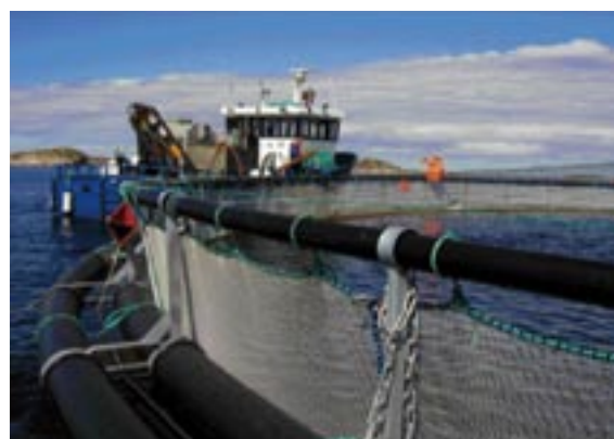
■ Figure 2.3 Specialised work boat operating a feed cannon on a plastic collar cage in Norway 10
