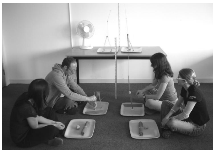
Fig. 1. The testing area. Participants were seated on the floor in front of a table, and built their towers on trays. A measuring tape ran from the floor to the tabletop, and then from the tabletop up the wall. Completed towers were moved from the floor, on their trays, to the tabletop. A desk fan was located on the tabletop, directed towards the towers.
