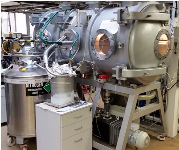
Fig. 2. The Large Mars Planetary Environmental Simulations Chamber (centre), vacuum pump (bottom), liquid nitrogen supply (left) and CO 2 gas cooler (front left of centre).
